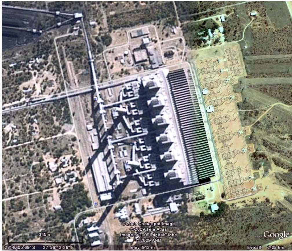
Fig. 6. Matimba Station, RSA, with ACCs to the right of the powerhouse; from Google Earth .
